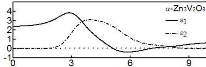
Figure 5 Real and imaginary parts of the dielectric function of  $\alpha\text{-Zn}_3\text{V}_2\text{O}_8$
