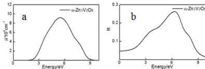
Figure 6 Absorption(a) and Reflection(b) spectrum curves of  $\alpha\text{-Zn}_3\text{V}_2\text{O}_8$
